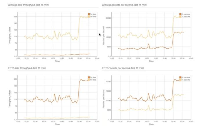
Additional tests showed that the link could operate at up to 240Mbps with over 210,000 packets per second, if needed.
